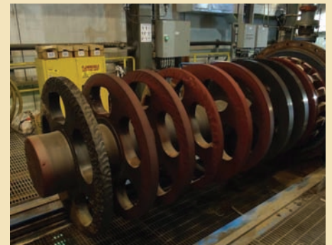
Grinding disks and rotor inside new M5000 Isamill.
